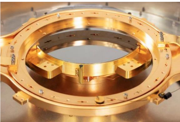
Wafer under probe card fixture
