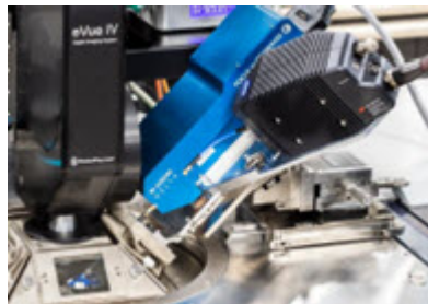
RFA-F110-EH-TH assembled on system
