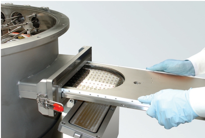
Loading of wafer / die carrier into the vacuum chamber.
