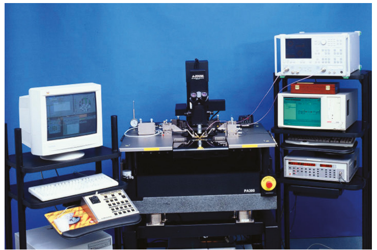
RF tests with IZI Probe® on PA300.
