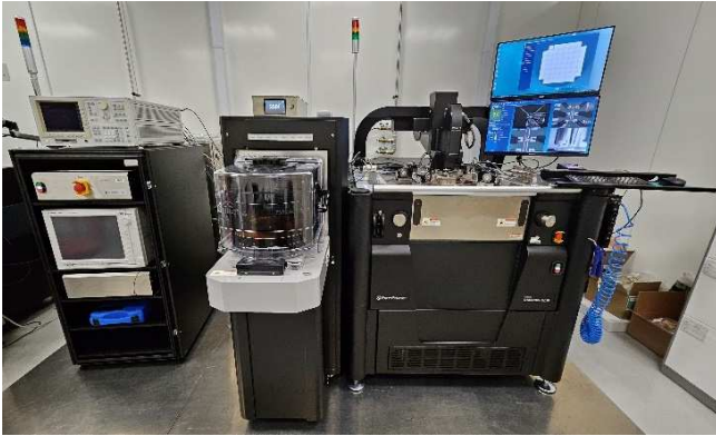
Fig. 4. 300mm fully automatic probe system with cantilever quasi-Kelvin QK and MEMS true-Kelvin TK (b) probes for wafer-level device characterization.
