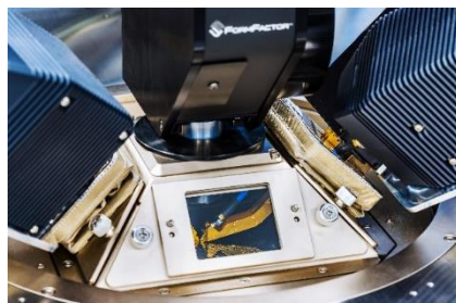
FormFactor T-Wave Dual band probe with integrated diplexer
