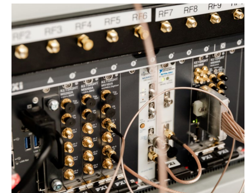
Figure 2. Electronics rack with Keysight PXI embedded controller and PXI modules used in the Model 106 Integrated Measurement Solution. Image courtesy of Seeqc.
