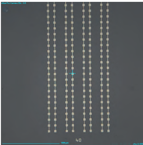
eVue V 10x and 40x Pro – 10X objective, 0.5 Zoom (40 \mu\text{m} pad)
