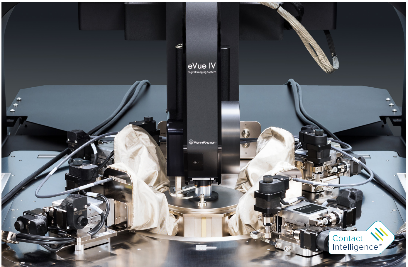
Motorized positioners with patented FlexShield enable highest accuracy in a dark, shielded and frost-free environment.
