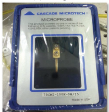
(b) True Kelvin DC probe with pitch 8µm, probe tip radius of 1.5µm
