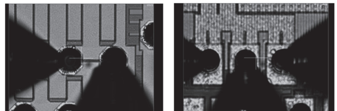
(a) 2-Micro-Bump Test Structure with 2 True Kelvin Probes (b) 3-Micro-Bump Test Structure with 3 True Kelvin Probes
