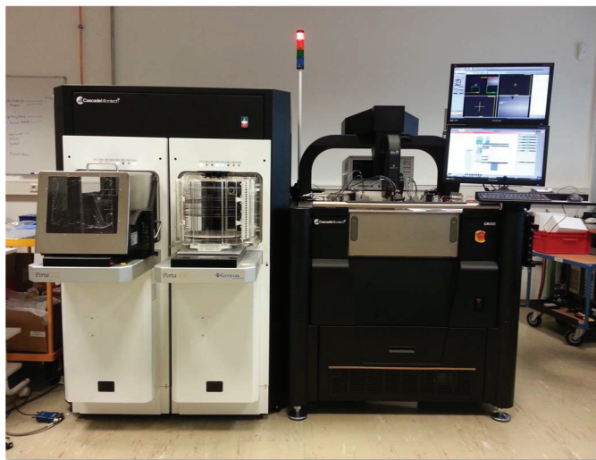
Fig. 5. Cascade Microtech CM300 Fully Automatic Probe System with 200mm and 300mm Wafer Load Ports and Keysight Semiconductor Parametric Analyzer.
