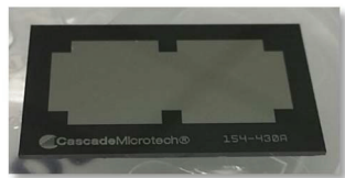
(c) Aluminium contact substrate to planarize the true Kelvin probe
