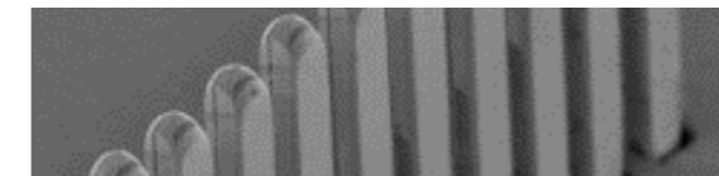
FormFactor low-force 2D MEMS MF spring family for 60 μm pitch pads applications.
