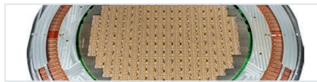
SmartMatrix™ enables parallel testing of >3000 DRAM DUTs on 300 mm wafers
